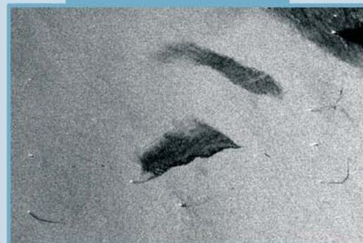
Natural slicks and oil spills, as shown in the SAR image left, have a smoother structure than the surrounding ocean and can be detected using Synthetic Aperture Radar.
